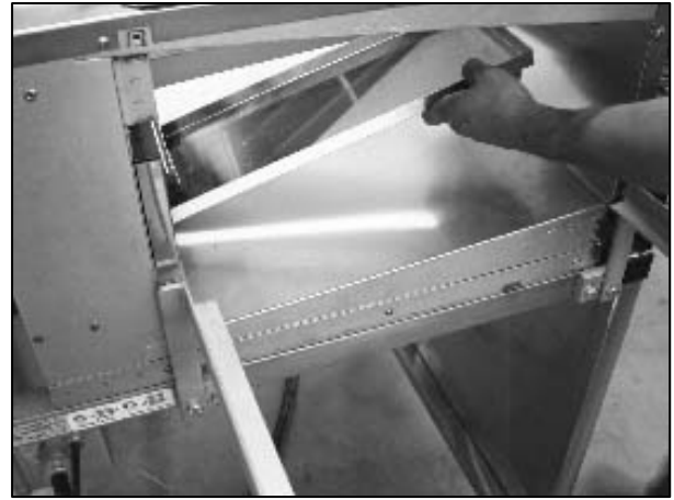
24. Remove the oven crumb tray
